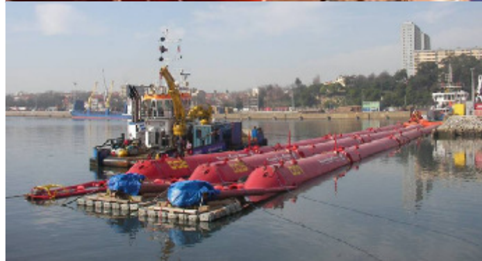
Location of the Aguçadora Wave park (left; Google Earth ). Constructions of the modules of power take off (top right) and three pelamis machines, 750 kW each (bottom right) in the harbour of Leixões, ready to be deployed ( Pelamis wave Power ).
